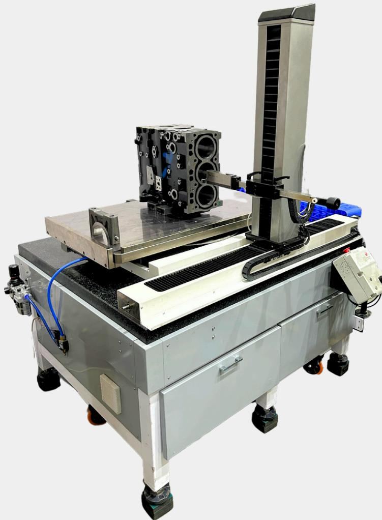
This machine is designed for precision measurement and machining applications with 5-axis movement capabilities. It is ideal for large-scale parts such as cylinder blocks in automotive manufacturing or similar industries requiring high precision and flexibility. The machine offers flexibility with pneumatic locking and manual slide locks for added safety and versatility.
